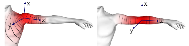
Figure 4: Local coordinate systems and weights d_j of our joint-based deformers (here the shoulder and the elbow). © 2012 The Authors
