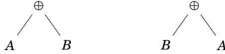
Fig. 3. The parse tree for the expression A \oplus B before (left) and after (right) a commutative transform.
