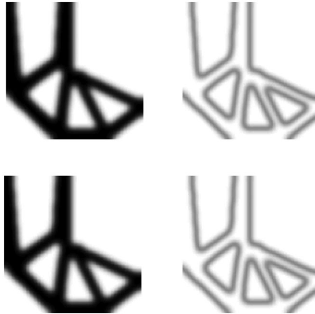
FIGURE 15 Mean (left) and standard deviation (right) of processed design variables \bar{\rho} obtained from biresolution optimization with a 10 \times 10 mesh (top) and single-resolution optimization of a 100 \times 100 mesh (bottom)
