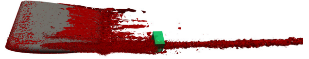
Fig. 13. 3D NACA wing case example of vorticity (before filtering). The box shown in the wake denotes the region within the field over which the results will be compared.
