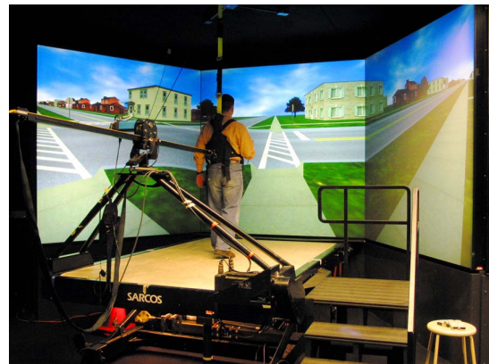
Fig. 1. Treadport Virtual Environment comprising a CAVE-like visual display and locomotion interface
