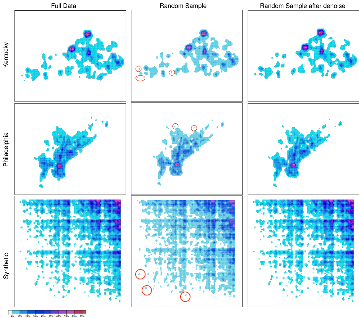
Figure 7: Visualization of random sample KDEs of all three datasets. Showing all isolevels of a random sample (middle) shows false anomalous regions, circled, compared to ground truth (left). After zapping process, (right) still preserves the rough shape of the data—enough to know where to explore more—without any of the false positive regions.
