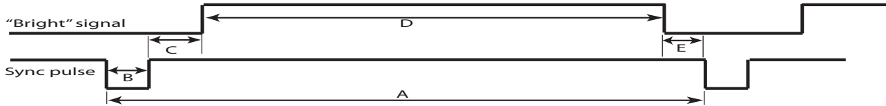
Figure 4: VGA interface signal timing
