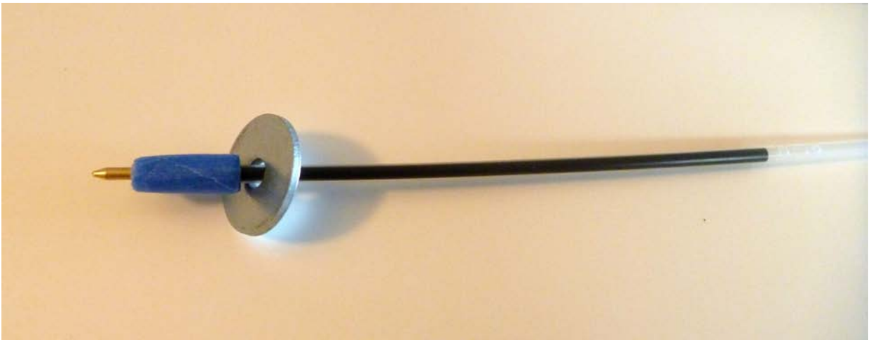
Figure 17: I need a flat surface for the foam core to pivot on. I've made a "shelf" using masking tape, and then put a fender washer (a washer that is a little larger in diameter than a standard washer) on the pen. The foam core will ride on top of this fender washer.
