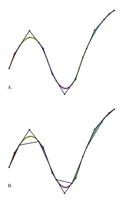
Figure 22: A refined curve provides a separate convex hull for each seed point. (A) The interval associated with each seed point colors each portion of the curve. (B) The refined control polygon produces tighter convex hulls that more closely bound the seed points.
