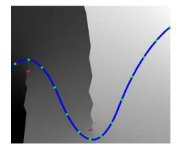
Figure 20: Choosing a seed point that converges only to a local minimum produces the zigzag pattern along the medial axis of the curve.
