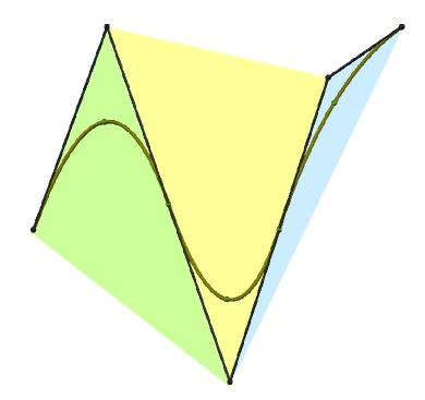
Figure 21: This quadratic curve has three polynomial pieces. The convex hull for each piece is shown as a different filled region. Each convex hull can enclose multiple seed points.
