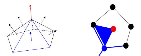
Figure 42: A. The vertex normal is surrounded by triangles. B. Each triangle normal maps to a point on the Gauss sphere and each edge maps to an arc.
