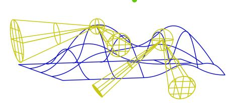
Figure 31: Two surface patches with their sample tangent cones. The spheres bound he spatial extent of the patch and help to form the solution line cone from the query point.
