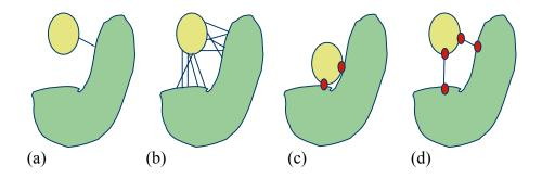
Figure 48: Different distance possibilities for force computation. (a) The global minimum distance. (b) All pairs within a distance. (c) Contact points between two colliding models. (d) Local minimum distances.
