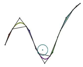
Figure 23: The circle shows the current upper bound on distance. The convex hull at the bottom of the curve overlaps that circle, showing that its seed point may produce a new global minimum.
