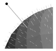
Figure 39: The line between the query point and the feature is in line with the normal at the feature.
