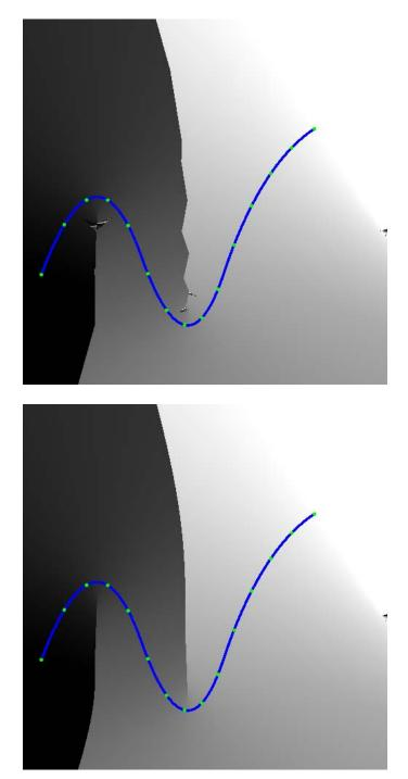
Figure 24: Distance fields computed using a single seed point and using lower bound pruning. (top) Only using the closest seed point yields incorrect global minima. (bottom) The lower bound pruning technique developed in this chapter produces global minima as well as improved convergence.
