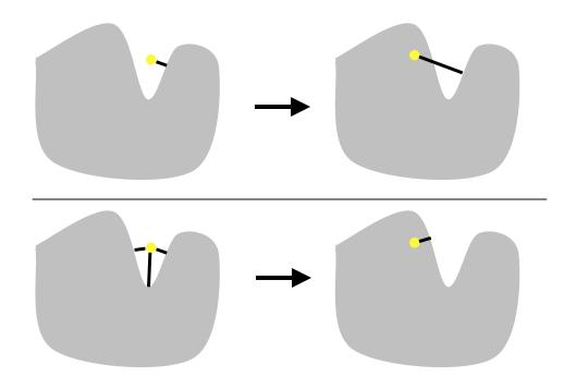
Figure 36: All local minima are needed to initialize local tracking. (top) A global minimum is not updated in time to jump the local tracking to the new side. (bottom) Normal cone computation finds all local minima, all of which are tracked, so the penetration is detected.
