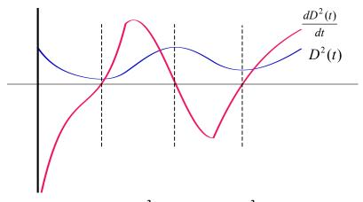
Figure 3: The derivative of  $D^2(t)$  overlaid on  $D^2(t)$ . Zero crossings correspond to extrema in distance.
