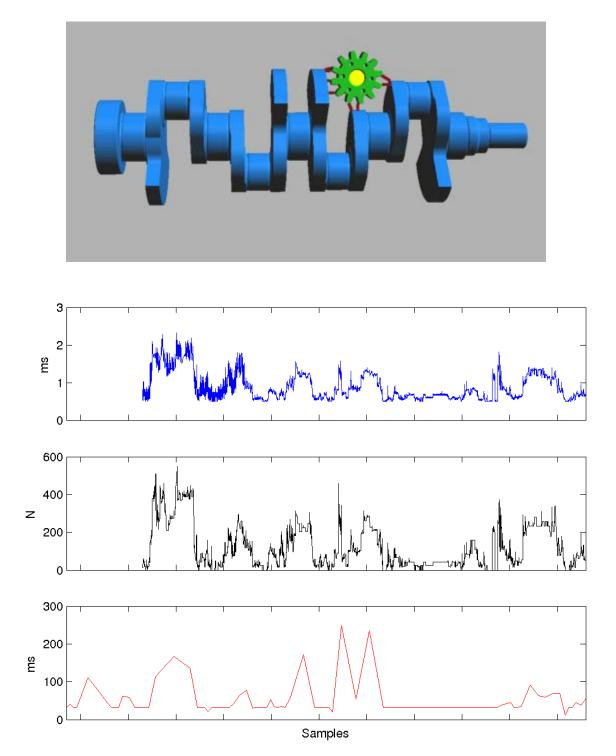
Figure 57: The crankshaft model has 45,000 triangles and the gear has 6,300 triangles. The local update time correlates well with the number of triangles searched. The bottom graph shows the computation time for the global search to find the LMDs. Without the local update, haptic interaction would have been unstable and slow.
