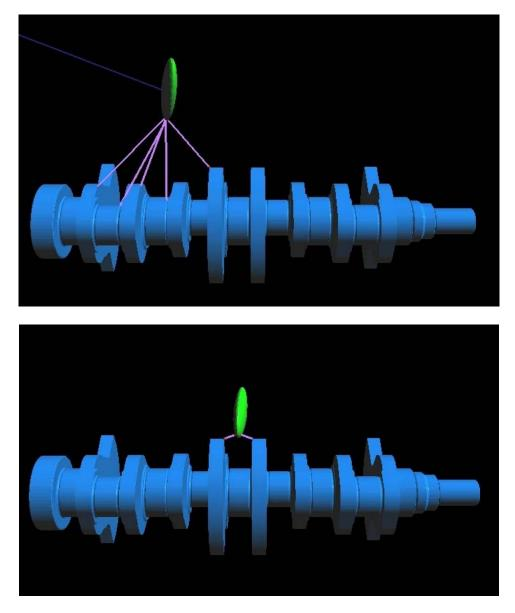
Figure 49: Finding all LMDs will create forces between far apart portions of the models, as shown in the top image. Using a small cutoff distance in the lower image removes unnecessary LMDs from consideration and controls the onset of forces.
