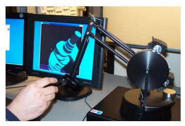
Figure 47: The 6-DOF Phantom used in a virtual prototyping session.
