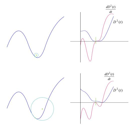
Figure 4: As the query point moves away from the curve (left column), the squared distance function (right column) changes from a minimum to an extremal distance at the same zero crossing of the derivative function.
