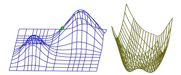
Figure 5: The squared distance between the point and surface at left is visualized on the right as a function mapping parameter value vs. squared distance.
