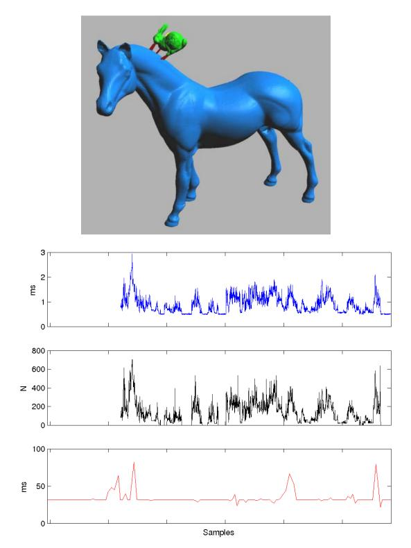
Figure 59: The horse model has 97,000 triangles and the bunny model has 2,200 triangles. The finely detailed surfaces can produce nearly redundant local minima. In this example, the algorithm still updates the LMDs and forces at around 1 kilohertz.
