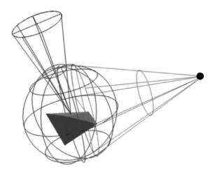
Figure 41: A node of the SNCH contains geometry bounded by a sphere. The range of vectors from a query point to that sphere forms the solution line cone, which bounds the range of vectors to the contained geometry.
