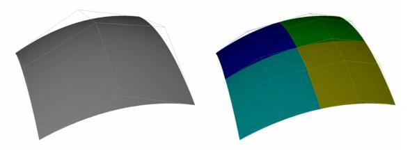
Figure 32: Refining a patch splits it into four independent surfaces. The new control meshes more tightly bound the surface.
