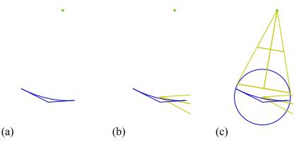
Figure 25: Building the bounds on normal and solution vectors.(a) The query point and curve interval, with its control polygon.(b) The tangent cone computed from differences of control points.(c) The solution line cone encompasses the circle around the interval.
