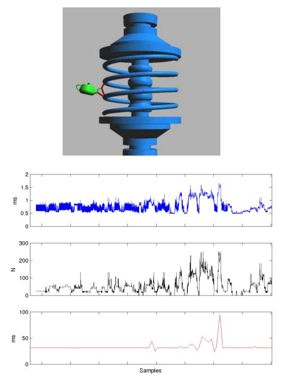
Figure 58: The spring model has 23,500 triangles and the teapot has 5,600 triangles. Even though the models are high resolution, typically there were only a few LMDs to track, and the local update was able to maintain a high update rate.
