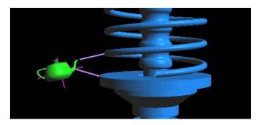
Figure 46: The SNCH approach finds local minimum distances between models and applies repulsive forces to prevent contact.
