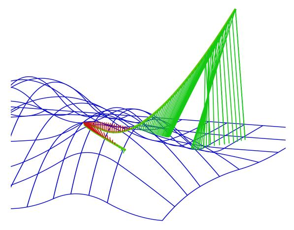
Figure 37: A simulated haptic path enters a surface. Above the surface, multiple minima are tracked, whereas only one is tracked while below. Forces are generated only while inside. The normal cone computation updates the set of local minima for the local update to maintain at haptic rates.
