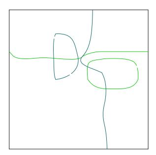
Figure 6: The zero crossings of each partial of the distance-squared function generically form curves in the *uv* plane. The intersections between the two curves are local extrema of the distance-squared function.
