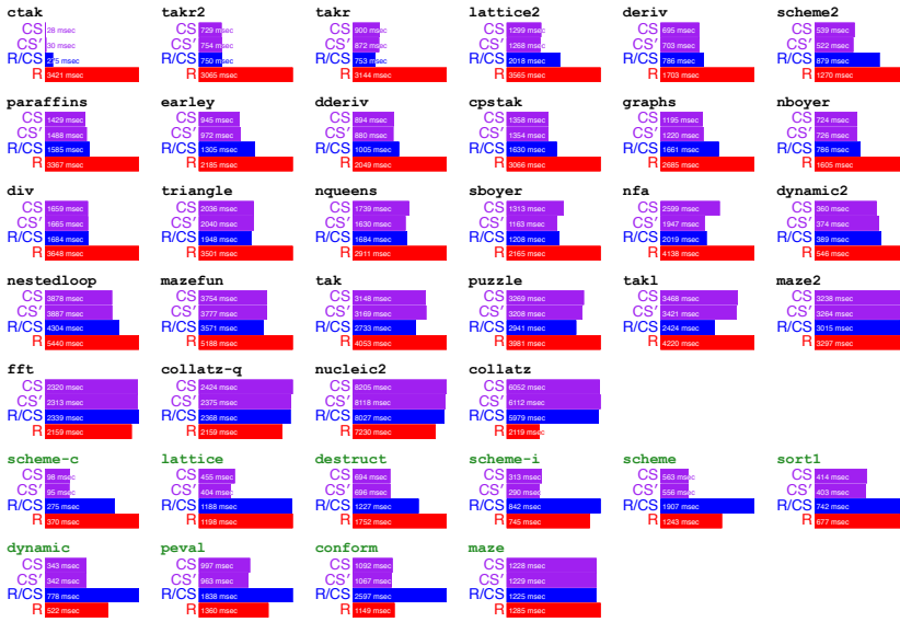
Fig. 1. Traditional Scheme benchmarks. Shorter is better. CS = unmodified Chez Scheme, CS' = modified Chez Scheme, R/CS = Racket CS, R = current Racket implementation.
