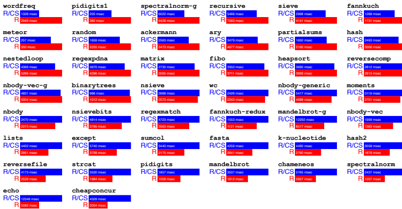
Fig. 2. Shootout benchmarks. Shorter is better. R/CS = Racket CS, R = current Racket implementation.
