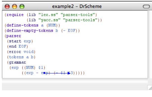
Figure 10 Correlating an action with the grammar
