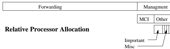
Figure 1: Hierarchical breakdown of the resource subdivisions of a hypothetical MCI router.
