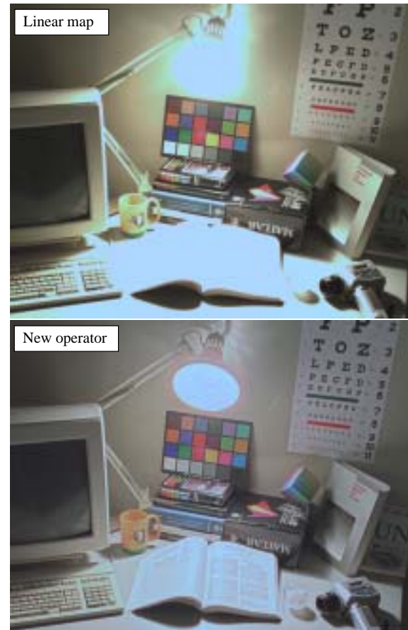
Figure 1: A high dynamic range image is difficult to display directly without losing visible detail as shown by the linearly mapped image (top). Our new algorithm (bottom) is designed to overcome these problems.
