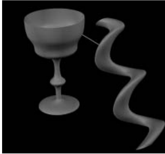
FIGURE 1. Finding the minimum distance between two parametric surfaces.
