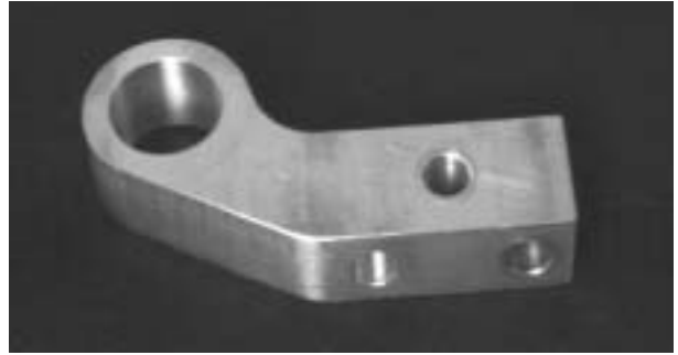
Figure 9: Steering arm: original part.
