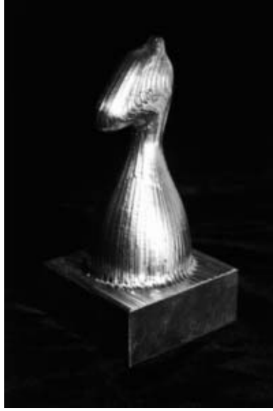
Figure 5.5. Aluminum milled version of the knight model.
