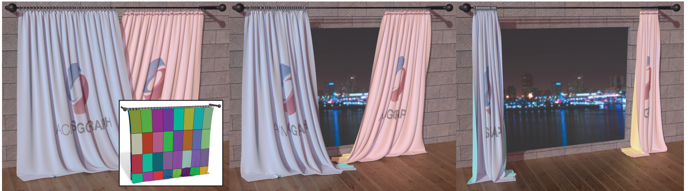
Fig. 19. Open the window. We show a high-resolution simulation involving 6M DOFs. Each curtain has 32 domains as shown. They are pulled away from the middle to reveal the view of a city night. At this resolution, inexact global solve will significantly increase the total number of L-G iterations (e.g., as in [Wang 2015]). Our method converges more effectively and uses 6.6 s to simulate one frame under h = 1/120 .
