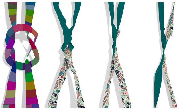
Fig. 16. Comparison with PD-IPC (GPU). Two fabric strips are tangled and pulled in opposite directions to form a tight knot. The left figure illustrates the domain partition in the rest configuration. Similar to PD-IPC, we apply the CCD filtering after each iteration of the contact-aware global solve. There are 324K DOFs in the scene, and 57K collision constraints. Our method is comparable with PD-IPC, and runs at 564 ms per frame. The runtime performance of PD-IPC for this simulation is 544 ms per frame. The time step size is h = 1/120 .
