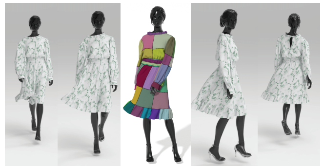
Fig. 17. Comparison with PD-EXP (GPU). In this example, we compare our method with PD-EXP [Lan et al. 2024] to simulate a virtual fashion show, where the character in a light midi skirt walks to the front and then turns around. We apply an external wind field to the left to generate more dynamic garment movements. There are 1.1M DOFs in the simulation. Due to the subspace pre-conditioning, PD-EXP is faster than our method. It uses 734 ms to simulate one time step ( h = 1/120 ), while our method needs 1.06 seconds on average.
