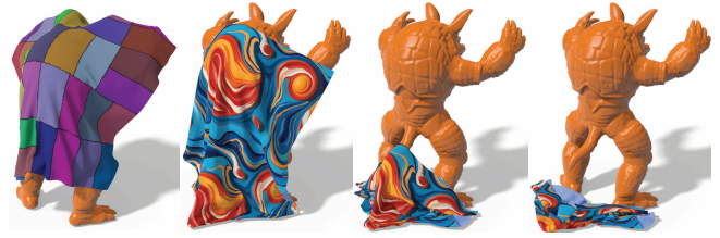
Fig. 14. Comparison with PD-Coulomb (CPU). Our method is faster than PD-Coulomb [Ly et al. 2020] by an order. In this experiment, a piece of cloth drops on an Armadillo and falls on the floor. While PD-Coulomb is also accelerated by CPU multithreading, the parallelization only applies at the local projection with OpenMP. Our method can be better accelerated by more CPU cores at both local and global steps, and it also converges faster than PD-Coulomb due to our novel projection scheme. In this experiment, there are 282K DOFs, and our method uses 145 ms to simulate one time step.
