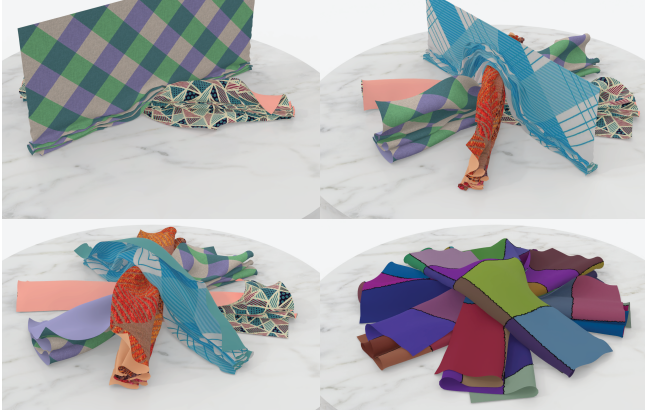
Fig. 20. Folding. In this scene, four tablecloths fall on the table one by one with different orientations. When stacking on each other, complex self-collisions are generated. Our method can robustly handle this simulation. There are 492K DOFs in the system, and the simulation runs at 557 ms per frame.
