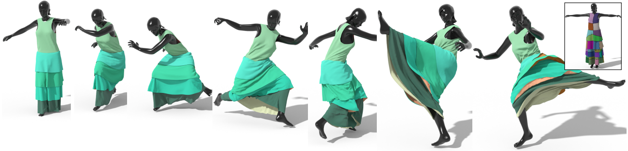
Fig. 15. Comparison with PD-BFGS (GPU) & C-IPC (CPU). The character in a tired skirt performs a kicking action. Fast body movements generate interesting garment dynamics and rich self-collisions. There are 444K DOFs in the scene. All the methods produce high-quality animations. Our method uses 588 ms for solving one time step ( h = 1/120 ), which is 2.6\times faster than GPU-based PD-BFGS and 66\times faster than CPU-based C-IPC.
