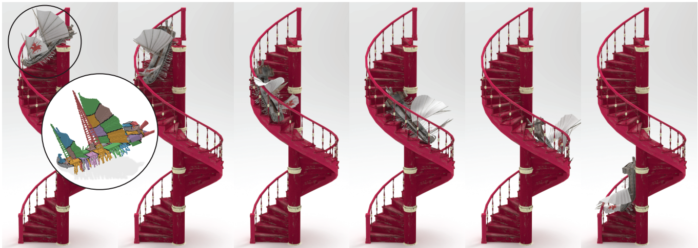
Fig. 23. Barbarian ship on the stair. In this example, the barbarian ship slides down on a spiral stair. There are 487K tetrahedron elements on the ship, which is decomposed into 64 domains. Our method uses 379 ms to simulate one time step, which on average needs 10 L-G iterations.
