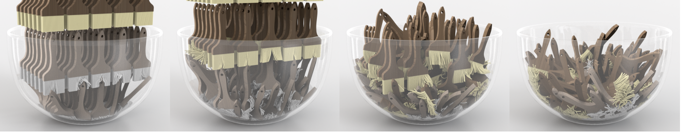
Fig. 10. A lot of brushes. There are 140 brushes dropping into the bowl under gravity. The yellow bristles are 20× stiffer ( E = 10^7 Pa ) than the grey ones ( E = 5 \times 10^5 Pa ), while the handles are nearly rigid (wooden, E = 10^9 Pa ). Such a heterogeneous system is beyond the capability of regular block descent-based methods like VBD. JGS2-GQ offers better robustness than the vanilla JGS2, and it remains highly efficient without training. In this example, all the collisions are resolved at each time step using IPC, and our method is 5× faster than GPU-IPC [Guo et al. 2024], and 100× faster than PD-IPC [Lan et al. 2022b]. The convergence comparison is reported in Fig. 11.
