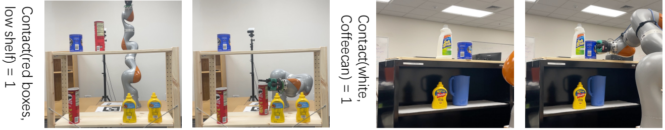
Fig. 10: Real-world evaluation with different shapes of shelves and different numbers of objects. Our framework achieves goals such as picking and placing an object onto different layers of the shelf and pushing several objects to make contact with one another in a shelf environment.
