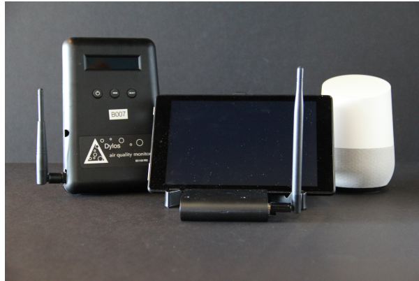
Fig. 1. Elements of a MAAV deployment. From left to right: a wireless Dylos air quality monitor, tablet display, Google Home and Raspberry Pi gateway computer (front). Wireless connectivity allows distributed instrumentation throughout participants' homes. Each deployment received three air quality monitors but is capable of instrumenting many more.
