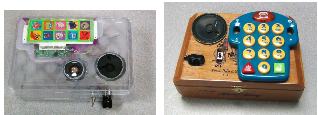
Figure 5: Noise-making toys modified by students through circuit bending / hardware hacking. The modified toys have been repackaged into new cases and new controls have been added.
